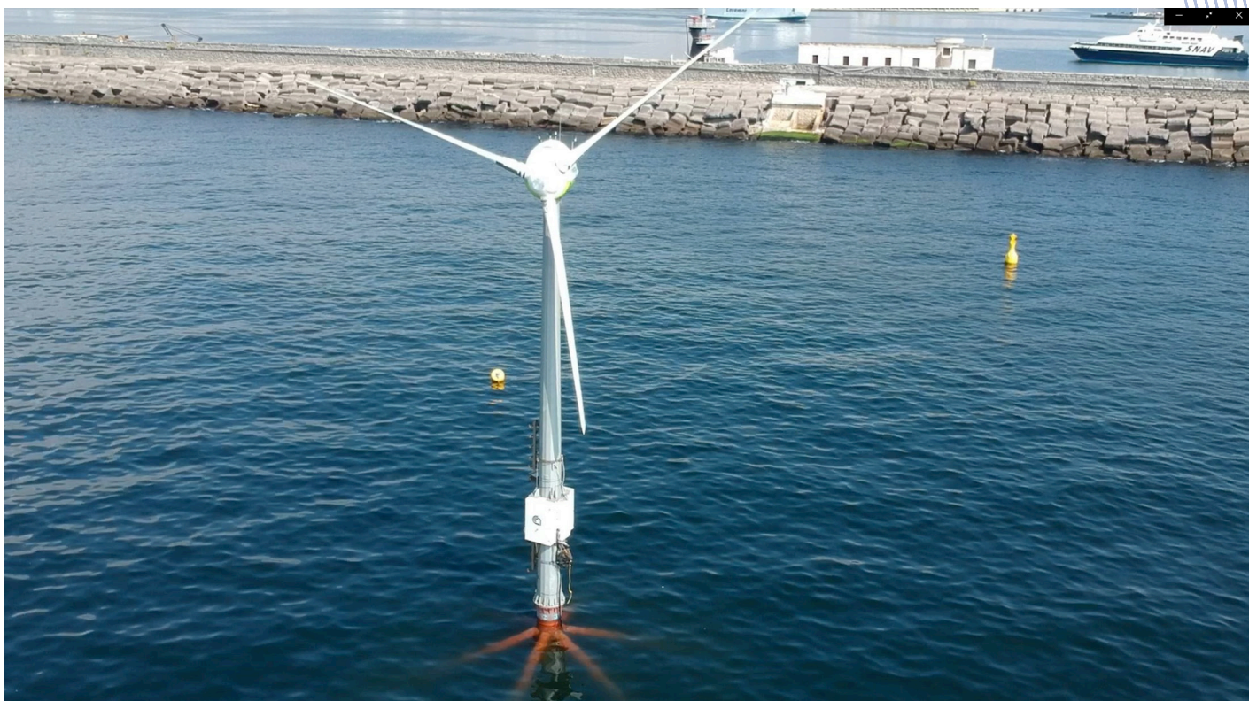
Prototype “Hexafloat” (Saipem floating wind turbine) at the MaRELab (Marine Renewable Energy Laboratory)
