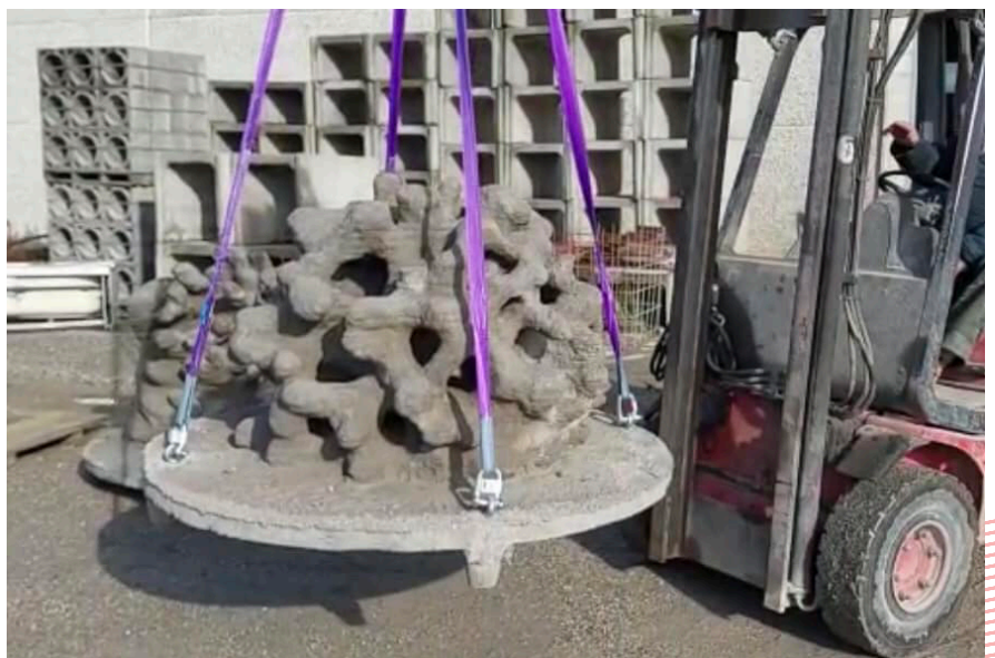
Figure 3. 3D Printed Reef by D-Shape, Enrico Dini. Project by Rossella Siani.
