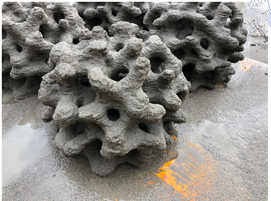
Figure 2. 3D Printed Reef by D-Shape, Enrico Dini. Project by Rossella Siani.
