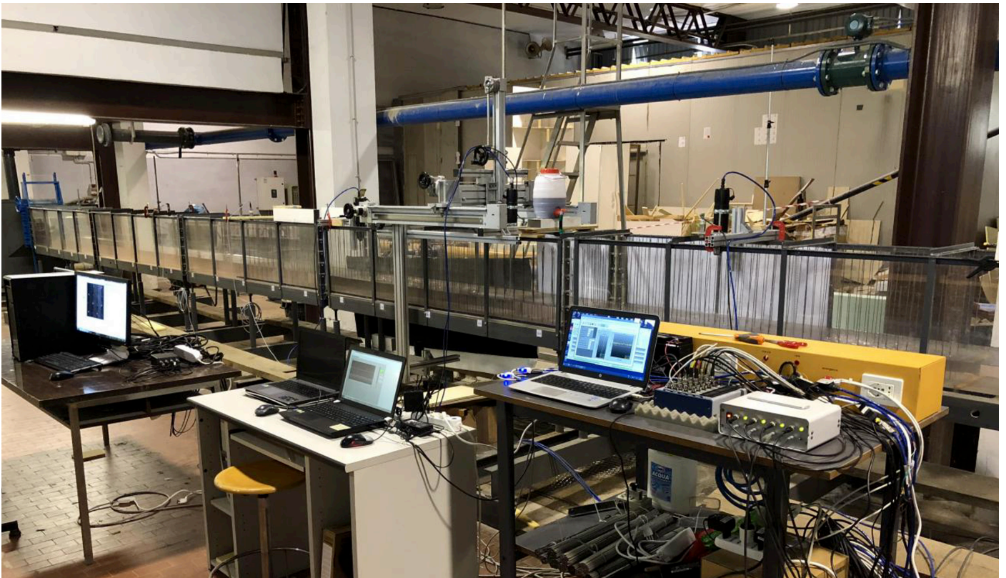
Figure 2. Picture of the channel where an experimental simulation of wave dumping due to rigid vegetation has been carried out.
